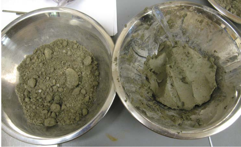
Photo 1: Soil sample with Portland cement before (left) and after (right) adding water.
