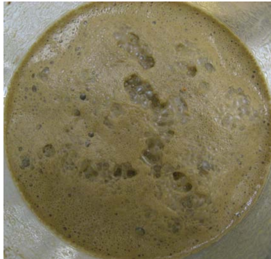
Photo 7: Top view of the foam produced in BT-3 as a result of gas generation.
