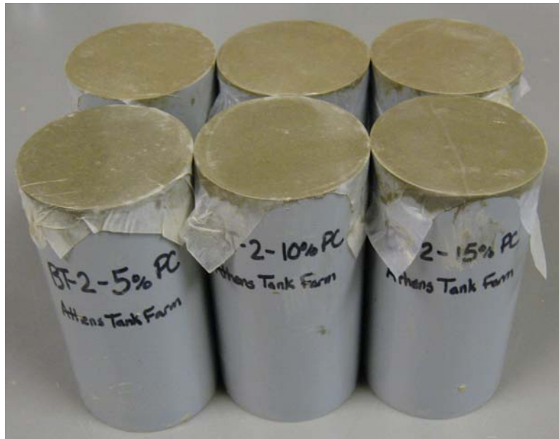
Photo 2: Stabilization test cylinders at t=0 with primary Parafilm® covering. A secondary covering of aluminum foil was then added.
